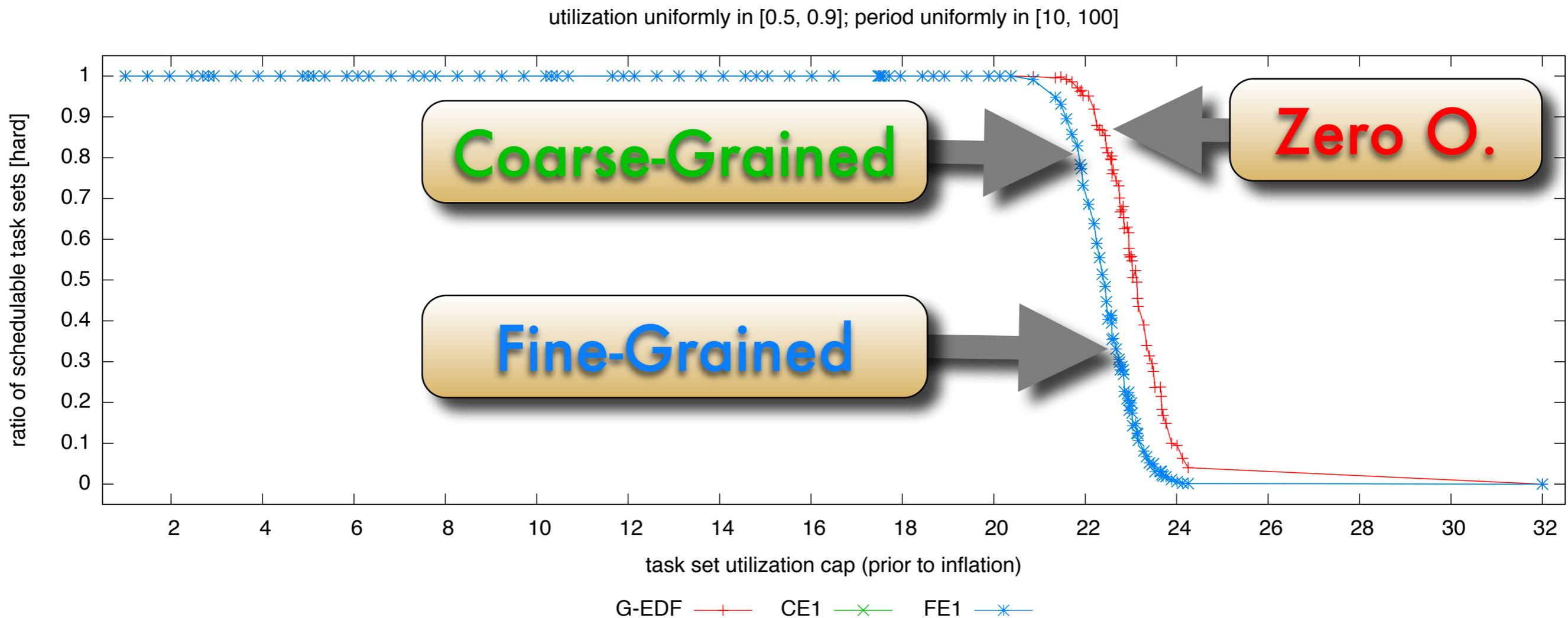
The **fine-grained ready queue** performed marginally better than the coarse-grained queue if used together with **dedicated interrupt handling**.
